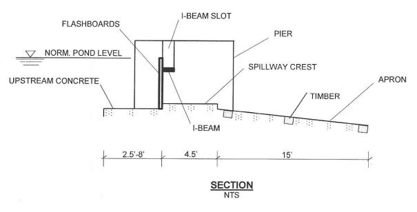
FIGURE 1. PISECO LAKE OUTLET DAM: PLAN AND SECTION
